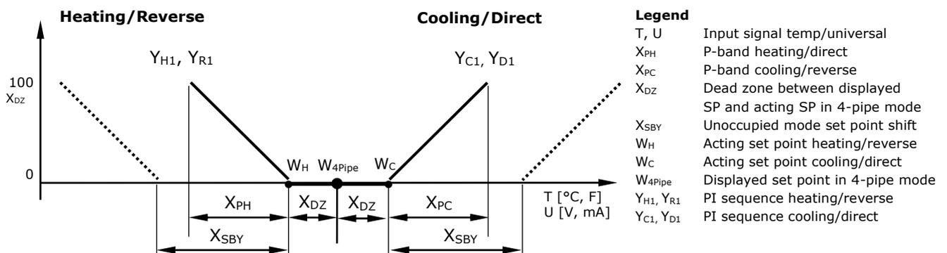
**New Feature: Switching binary outputs based on PI sequence:**
