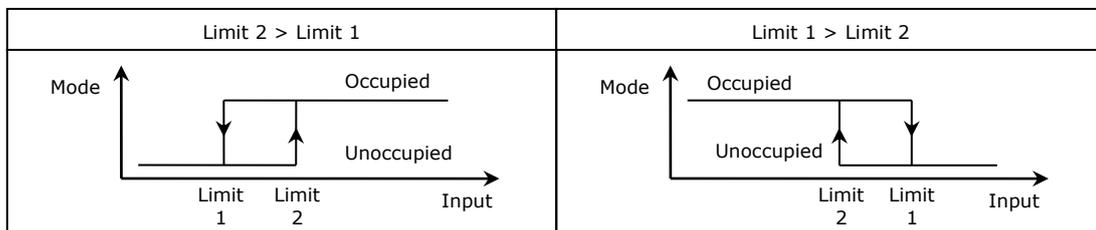
**3Fu Switch heating and cooling state based on input values**
