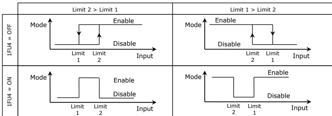
**2Fu Switch occupied and unoccupied modes based on input values**
