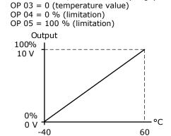
IP  $03 = -40 \, ^{\circ}\text{C}$ , IP  $04 = 60 \, ^{\circ}\text{C}$  (range)
